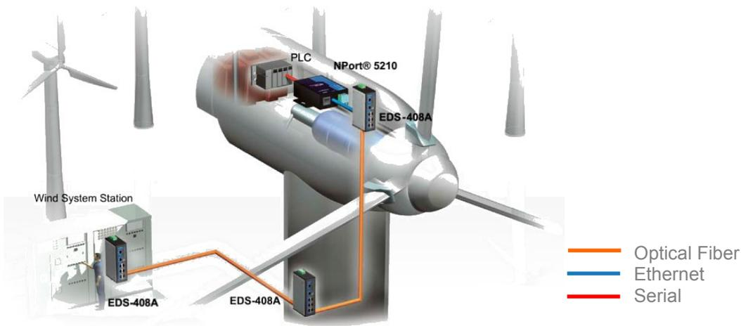
In this diagram the serial device server is playing its typical role, that is, converting the PLC’s serial data into Ethernet. The newly converted Ethernet “packets” are now routed to an Ethernet switch. Fiber optic cable serves as the data transfer medium that takes the PLC’s data to the wind farm’s control/operations monitoring center.
