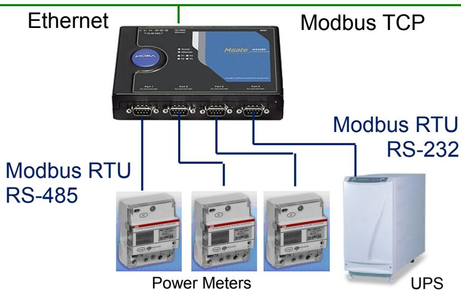
Observe how Modbus RTU RS-485 and Modbus RTU RS-232 field devices are interfaced to an Ethernet Gateway. The gateway in turn translates the differing protocols and sends it off as Ethernet “packets.” It’s good to have in mind that gateways are available with various serial port slots, making them ideal for several protocol distinct field devices, located in the same area, to be connected.
