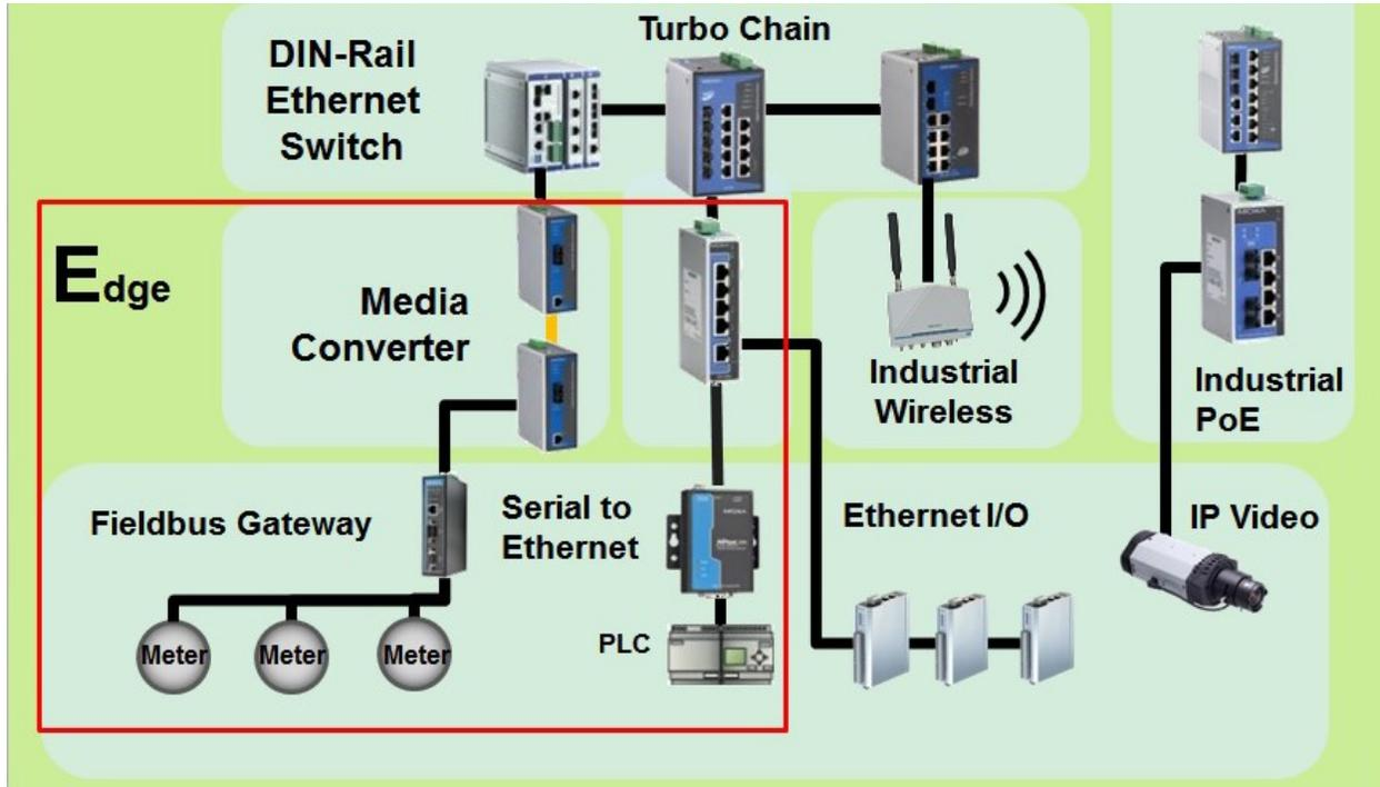
Note the bottom right corner of the squared (in red) section of the diagram. Connected to the PLC is an SDS. The Ethernet side of the SDS (opposite of PLC side) is connected to an Ethernet switch. We can now appreciate, from a hardware perspective, a serial device server's placement in an automation network. Once installed, the pertinent enhancements take effect, that is, converting the field device's serial data to faster, accessible, and ever-present Ethernet.
