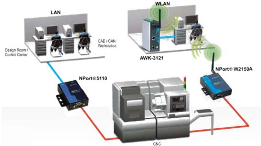
In this diagram we can note a SDS serving as the “middle-man” between this factory’s CNC machine, located on the production floor, and the plant’s control/operations monitoring office, which may/may not be at the same facility. What’s more, if we look at the SDS on the right side of the CNC we can perceive an implementation of a wireless SDS connected to a wireless Internet access point.
