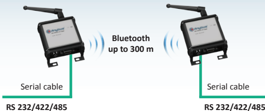
EXAMPLE 1: Point-to-point serial
