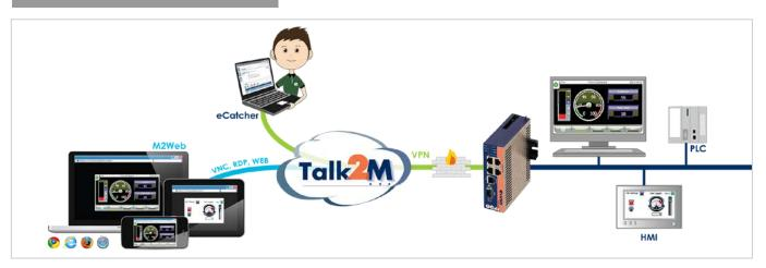
M2Web is a standard service of Talk2M, the secure cloud-based remote connectivity solution by eWON. M2Web provides easy and secure access to your remote site using the following technologies:
