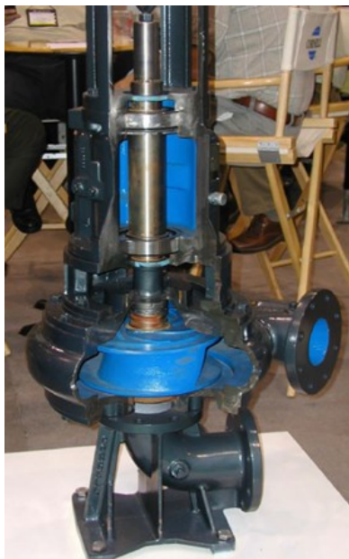
Figure 1 —Cut away of a Centrifugal Pump (Photo provided by: P. Hubbard, HRSD)
