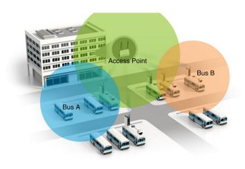
conflict avoidance system, CSMA-CA (Carrier Sense Multiple Access with Collision Avoidance), will fail. As a result, a high volume of packet collisions and retransmissions will overload the channel. Eventually, the access point, or even the entire wireless network, may temporarily fail under the load.
