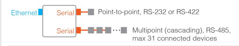
The NPort has 1 to 16 ports with interface option for RS-232, RS-422, or RS-485.
