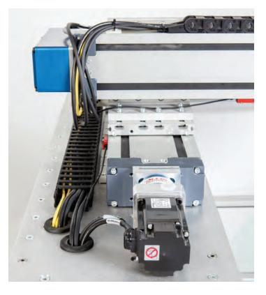
Box incorporates Rollon's TH series (TH 110 and TH 145) linear actuators. These compact, pre-loaded, ball-screw-driven units have zero backlash and offer positioning accuracy and repeatability within 5 µm.
