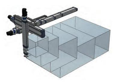
Motion Box has been fully tested with a 50 kg load at the edge of the motion envelope. The resulting deflection is no more than 1 mm. The initial system setup is already complete so that the end user can quickly and easily get parts moving in a reliable and repeatable manner. The time from pulling it out of the box to entering programming mode is roughly two hours. Regarding flexibility, six Motion-Box sizes are available to suit more than 80% of all Cartesian motion applications:
