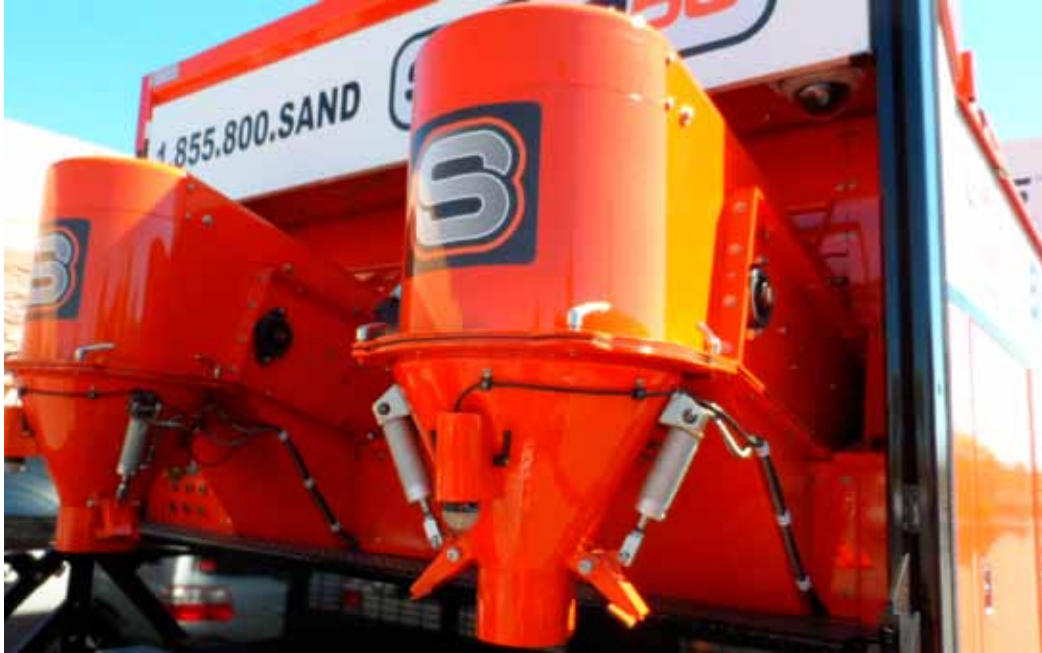
Figure 1: The Sandbags™ Super 50 has the ability to produce 2000 sandbags per hour. FEMA and local agencies have the ability to protect and save more lives and property with the advances made possible by the Sandbags™ Super 50 machines.
