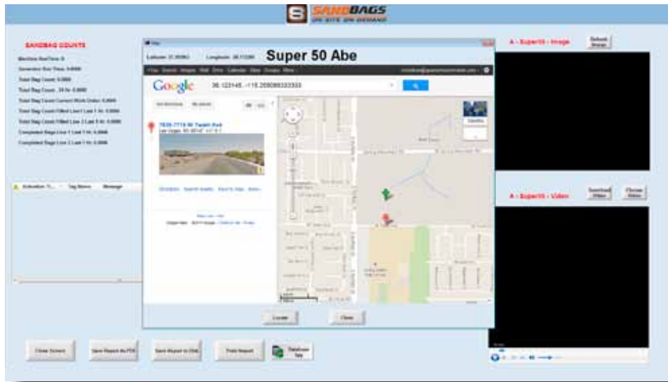
Figure 4: The application allows the sandbag machine to send GPS information and video back to central control.
